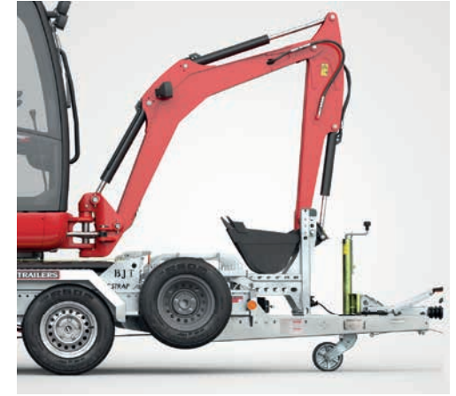
○ Digger Arm Lock Guides and secures the digger arm and bucket to the trailer with a single heavy duty locking pin.
